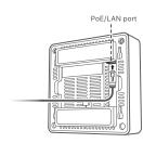
3 Connect the Ethernet cable to the
